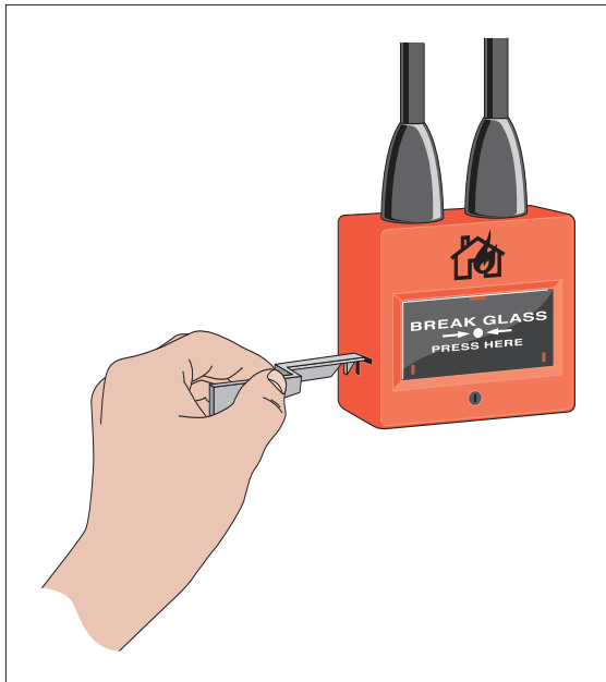
Figure 18: Using a test key
